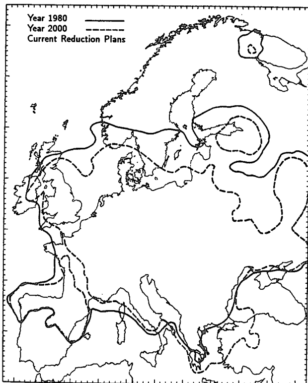
Fig. 5.7 Isolines of 1 \text{ gS} / \text{yr} \cdot \text{m}^2 for year 1980 and year 2000 under current reduction plans. Reproduced with permission from Alcamo et al., 1990 with permission.
