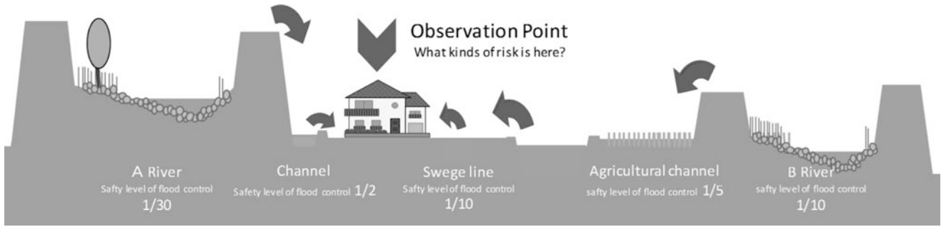
Fig. 13 Flood flow from various sources – facility safety vs. on-site risk
